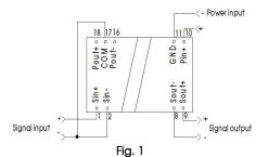
Note: Except for the case shown in application circuit two (Fig.b), pin 2 and pin 17 must be shorted when working.
