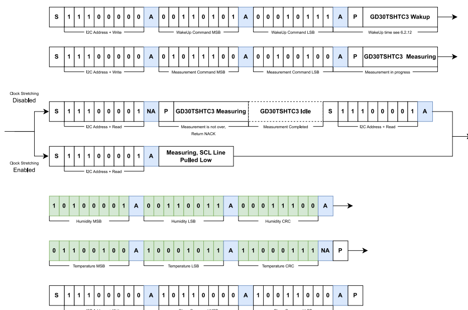
Figure 5. Wake-up, Start Temperature and Humidity Measurement, Temperature and Humidity Conversion and Sleep Command Execution Sequence Diagram
