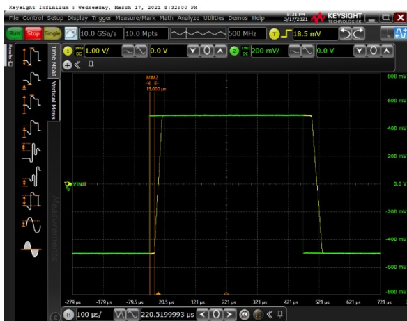
Figure 15. Overload Recovery at Negative Rail
