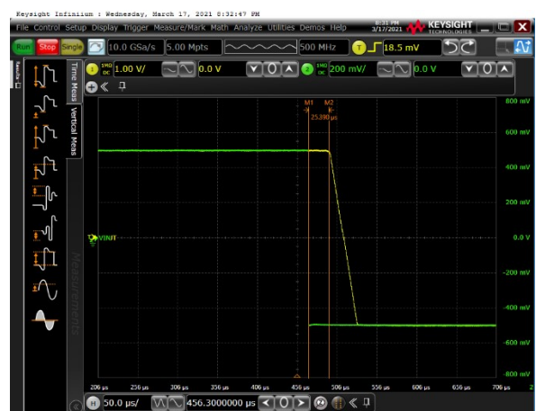
Figure 16. Overload Recovery at Positive Rail
